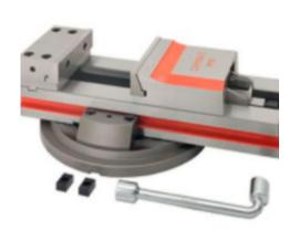
SPE81 ECONOMIC vices with oleopneumatic closure are called OSP81. A hydraulic cylinder inserted in the screw and an air-oil pressure multiplier ensure quick and safe clamping, without excessive work for the operator. The slide position can be adjusted by turning the screw with an ordinary wrench. The piece is clamped by operating the lever on the air-oil multiplier.
